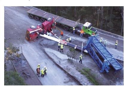
Figure 1: Articulated Crane Rollover when Carrying a Load [1]
