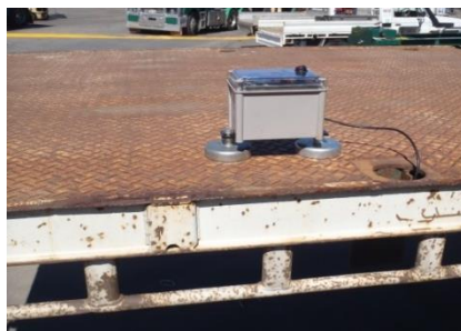
Figure 6: TMS Telemetry Hub to send Tyre Pressure / Temp Data
