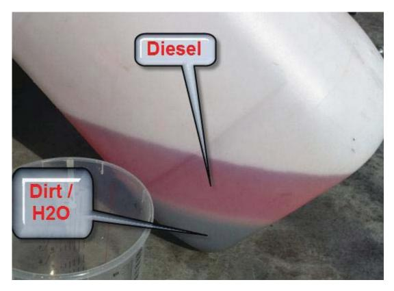
11. Drain the purifier and collect the substance (water, diesel, dirt) in a clean transparent can. When the fuel flow is clean you can close the ball valve.
