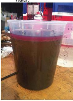
[Water =1,5 litre in purifier and 0.3 litre in the caterpillar separator. The rest (0.2 litres) is still inside the jerry can.]
