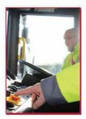
The VT StopSaf'e, effectively reduces the vehicle's speed while simultaneously bringing it to a controlled stop using the braking system. The system is activated using a secure emergency button installed to the vehicle dashboard, allowing the crew (or passenger) to react to an emergency situation.
